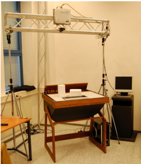
Figure 6: Two projectors mounted inside the table and on the ceiling are used in the IncreTable project. Moreover, the depth camera tracks the surface.
