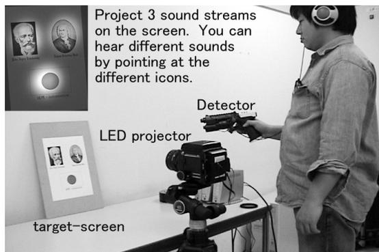
**Figure 13. Using primary LED projector**
