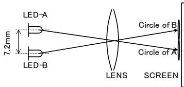
**Figure 11. Experimental set up using two LEDs**
