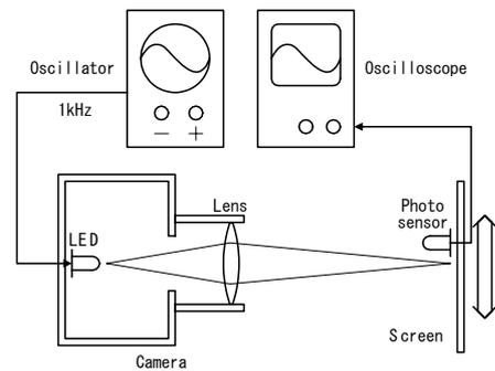
**Figure 8. Experimental setup using one LED projector**
