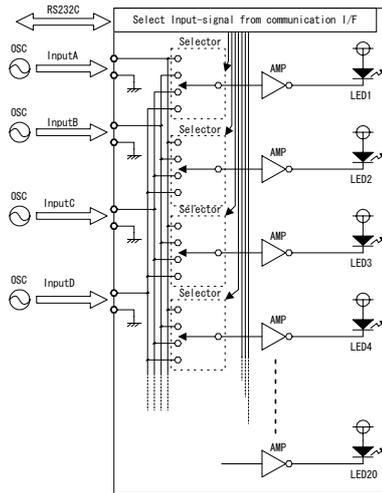
Figure 15. Block diagram of LED driver
