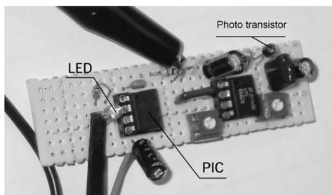
Figure 6. Close-up of a receiver
