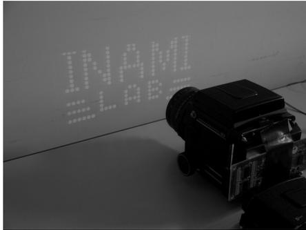
**Figure 7. Example of a LED projector**
