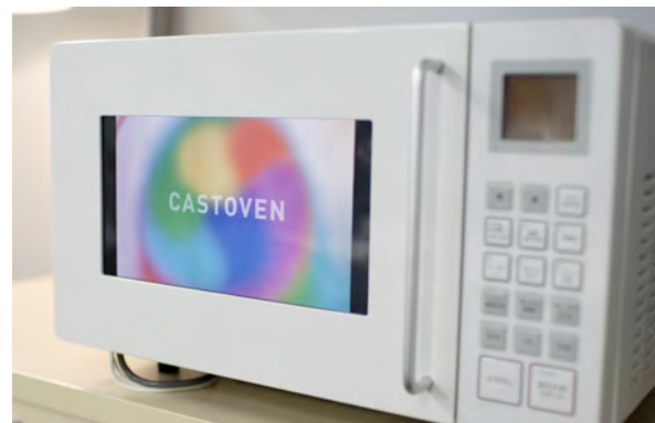
fig 2 CastOven is microwave oven with built-in LCD display on door. The system reads the cooking time from the control panel and retrieves a corresponding video from YouTube.
