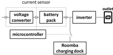
Figure 11. Parts on the Circuit Board of the Remote Dock.
