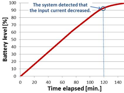
Figure 5. Constant Current Characteristic of the Appliance Battery.
