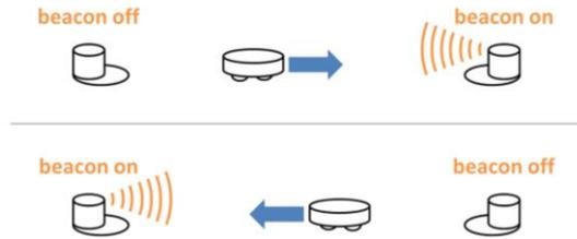
Figure 8. Time Division Switching of Robot Docks.
