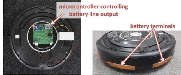
Figure 7. Battery-Charging Robot.
