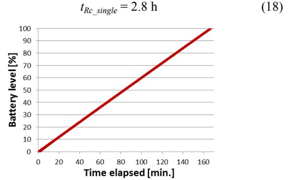
Figure 12. Constant Current Characteristic of the Robot Battery.
