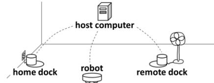
Figure 6. System Configuration.
