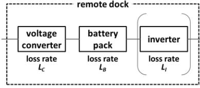
Figure 4. Energy Losses in Remote Dock.
