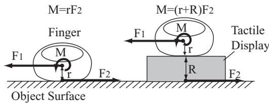
**Figure 5. Horizontal motion of the finger and generated torsional moment. F1: Finger force, F2: Friction, r: Distance between the center of the finger and skin, R: Display thickness, M: Torsional moment of the finger.**
