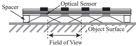
**Figure 7. Broaden the field of vision of the sensing element by mounting spacer on the sensor substrate.**
