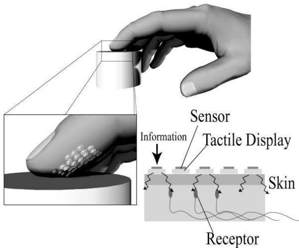
**Figure 2. SmartTouch: A new functional layer of the skin composed of a sensor and tactile display.**
