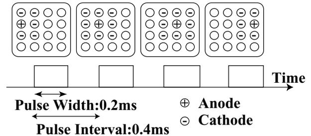
**Figure 12. Scanning procedure in cathodic stimulation mode [11].**
