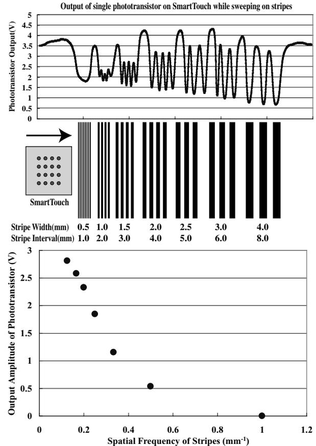
**Figure 8. Response of the phototransistor when sweeping on black and white stripes with different spatial frequencies.**
