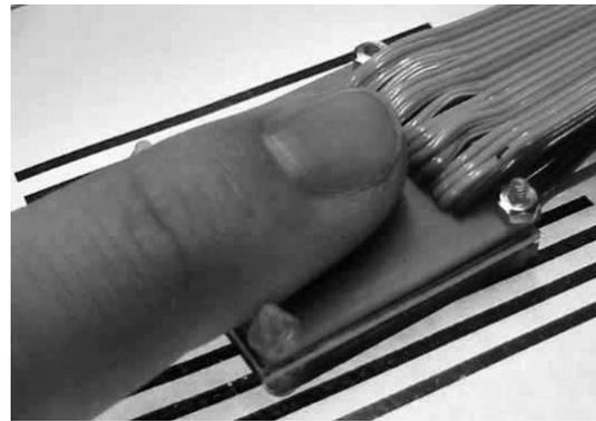
**Figure 3. Prototype of SmartTouch: Visual image (black and white stripes) is captured by optical sensors and displayed through electrical stimulation.**
