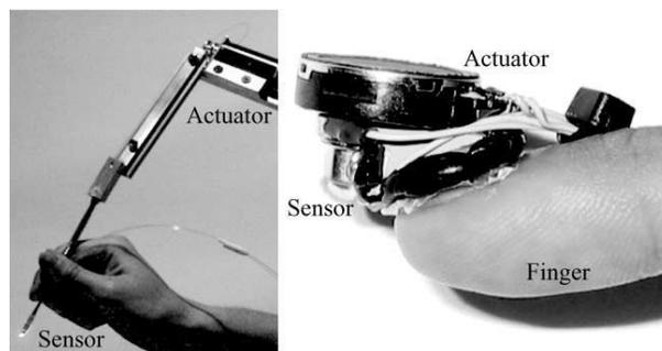
**Figure 1. Examples of Augmented haptics. (Left) SmartTool [14], (Right) SmartFinger [1].**
