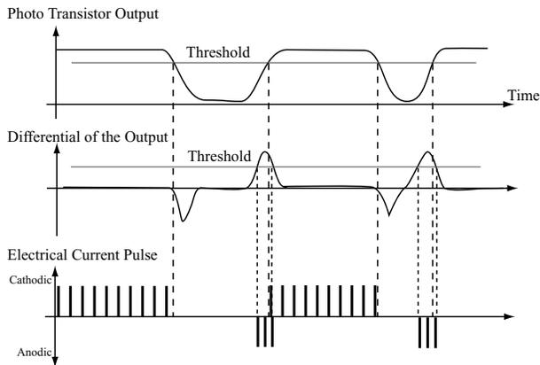
**Figure 11. Phototransistor output, its differential and electrical stimulation pattern of single electrode.**
