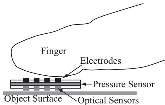
**Figure 4. Cross-section of prototype SmartTouch.**
