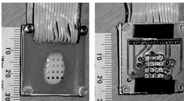
**Figure 6. (Left) Electrodes. (Right) Optical sensors. Both electrodes and sensors were arranged 2.5[mm]x2.0[mm] interval, 4x4 matrix. The position of each electrode was strictly aligned with an optical sensor.**
