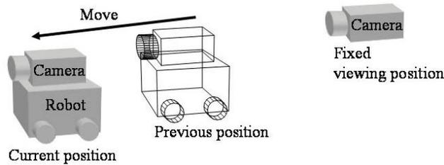
Fig. 4. Teleoperation using a fixed viewing position.
