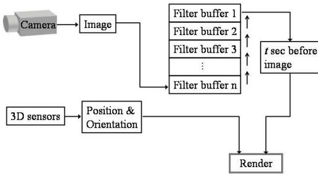
Fig. 7. Constant time delay image teleoperation.
