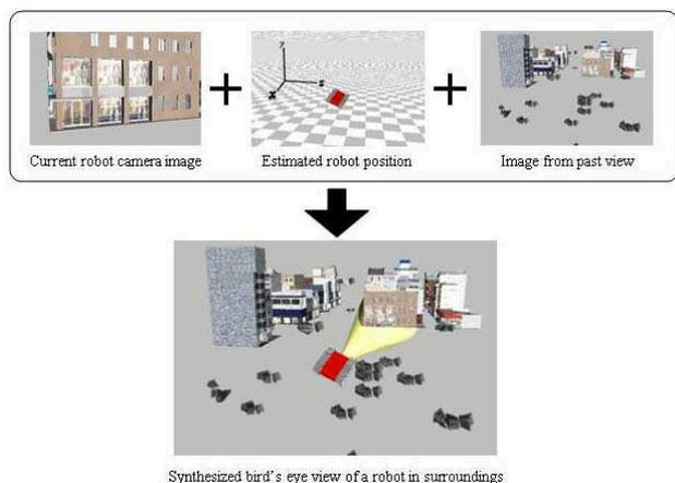
Fig. 1. Overview of the bird's-eye view synthesis.
