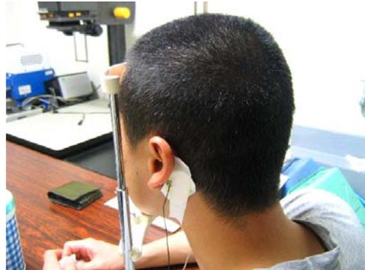
Figure 3. Electrodes applied to a subject.
