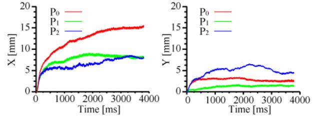
Figure 9. Displacement of Measured Points from Initial Position with High-Speed Camera at 600fps.
