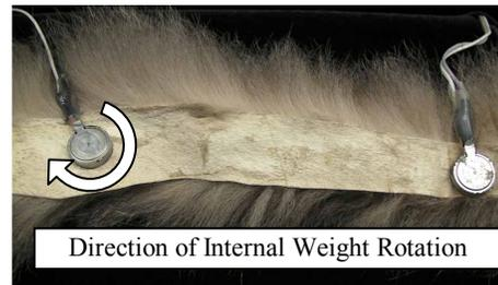
**Figure 4. Disk-shaped Vibration Motor To Provide Horizontal Vibration.**
