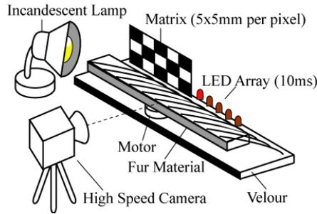
Figure 7. High-Speed Photography Setup
