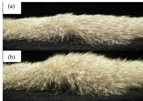
Figure 2. Bristling Effect with Horizontal Vibration Provided from Vibration Motor.
