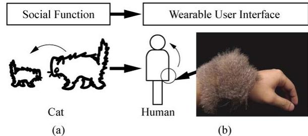
Figure 1. Soft and Flexible User Interface suitable for Wearable Computing Inspired by Hair Erection.
