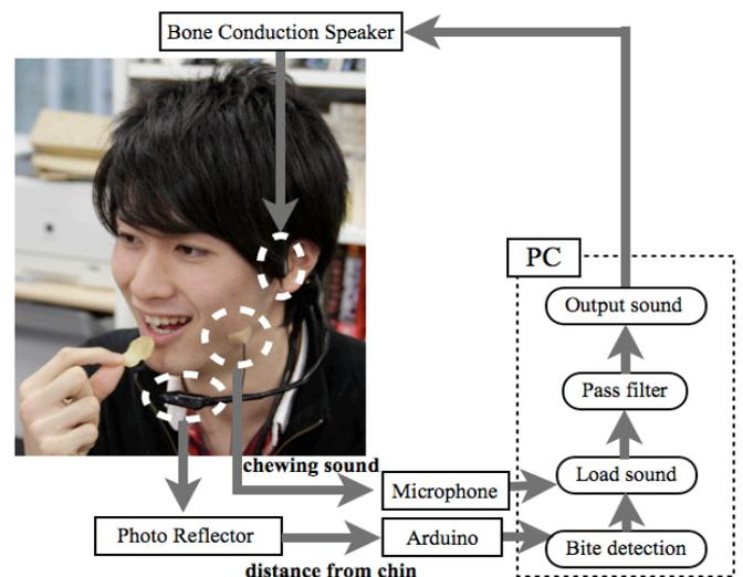
Figure 1. System block. This is a kind of feedback system. Human inputs the chewing sound and motion, computer outputs the suitable sound to feel augmented food texture.
